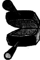
Tires are cured at over **300 degrees for 12 to 25 minutes**, depending on their size. As the press swings open, the tires are popped from their molds onto a long conveyor that carries them to **final finish and inspection**.
