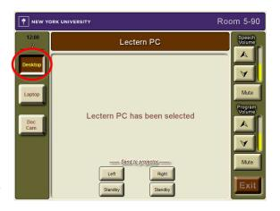
4. Once you've selected a device, press the **Left** or **Right** projector button at the bottom of the screen
