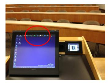
Projectors in this room are controlled by a touch-screen control panel
