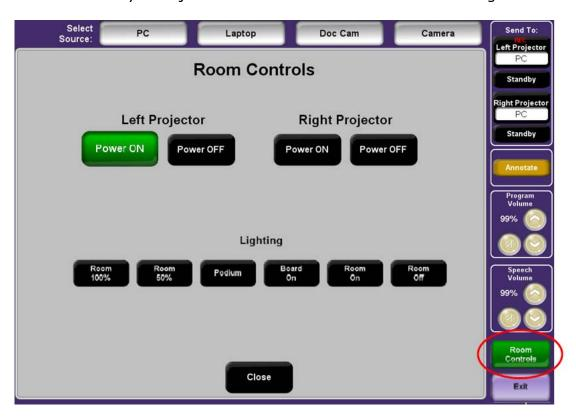
10. To power on or off any of the projectors press firmly the appropriate button on the screen. When you have pressed **Power ON** you will see a "warming up..." message on the screen.
