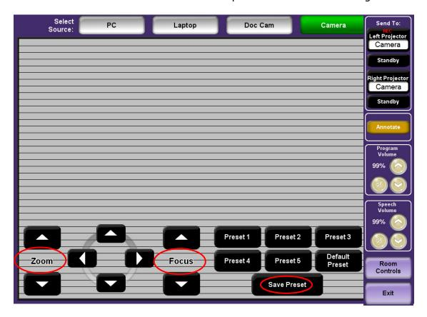
14. To Save a Preset do the following: Press **Preset1**, use the **Zoom** and **Focus** to get the desired view, and then press **Save Preset**.
