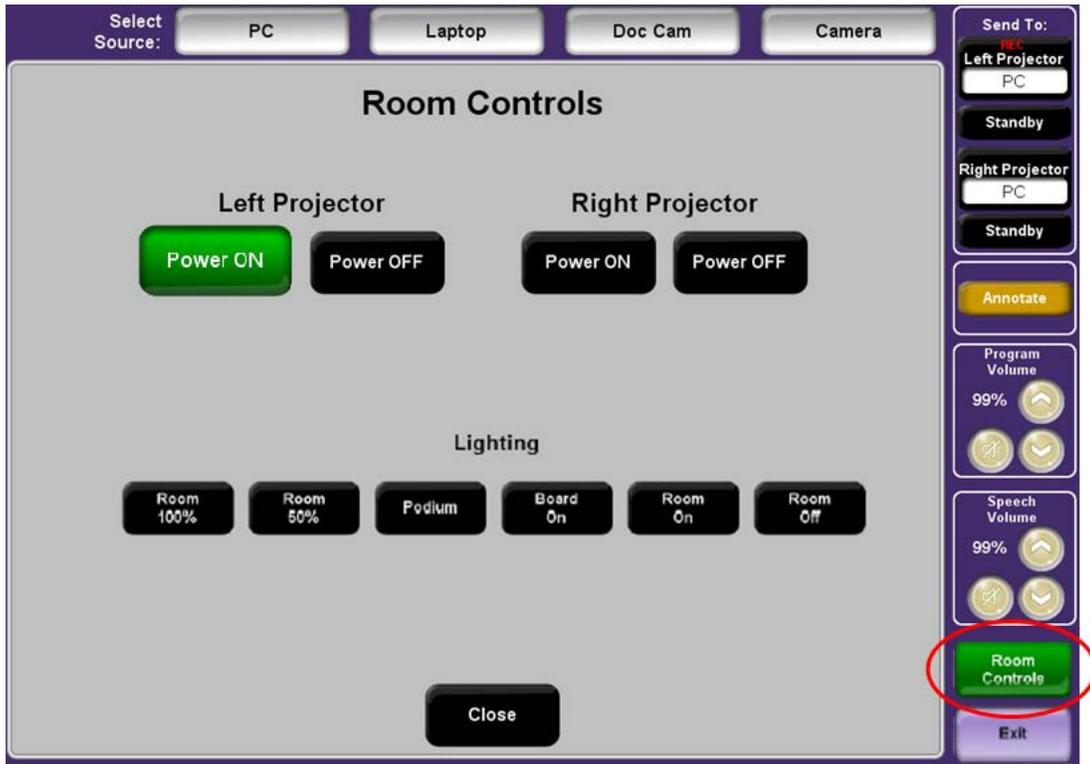
10. To power on or off any of the projectors press firmly the appropriate button on the screen. When you have pressed **Power ON** you will see a "warming up..." message on the screen.
