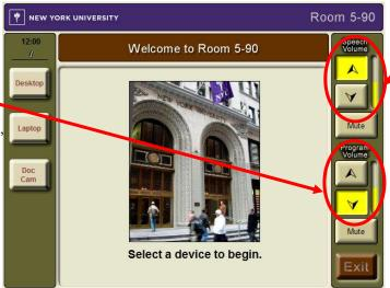
Volume controls the level of the lapel microphone worn by the instructor.
