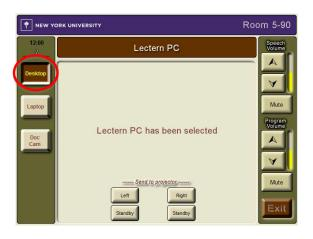
4. Once you've selected a device, press the **Left** or **Right** projector button at the bottom of the screen
